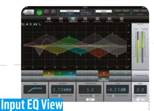
The Input EQ View accesses a comprehensive set of filter and delay functions that essentially duplicate the capabilities of the Output EQ section.
