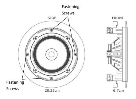
CS5 speaker can be mounted on the wall or ceiling.
