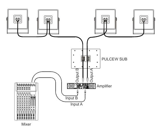
PULCEW mono instead has two NL4 speakon connectors in the connection panel referred as 'IN' and 'OUT'.
