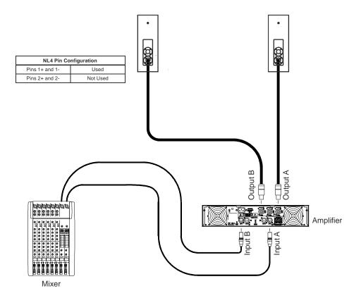
Recommended configuration in basic stereo system is represented below:
