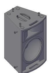
When installation is in suspended mode, use the upper or lower brackets. Unscrew one of the two screws hold a single bracket, the second screw must be screwed only after the first one has been tightened to avoid the bracket moves.
