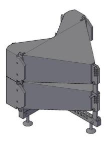
In case of installation in Flying mode, use the bumper without feet, attach the speaker to the sides via rigging holes, then connect the rear bracket adjusting the inclination.
