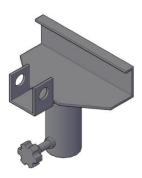
Install the bumper on the pole mount adapter, then secure them with the quick release pins.
