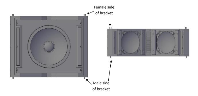
Overlap the speakers aligning the rigging holes, then secure them with the quick release pins.
