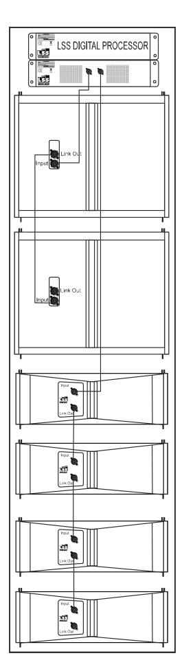
To use an array with ST17 and SB17 is necessary an external digital processor with custom setup provided by LSS. One output channel drive the SB17 and another one drive the ST17. If your amplifier can manage a 2 Ohms Load and has sufficient power, it possible to connect a maximum of 6ST17 in parallel per channel or 4 SB17 in parallel per channel (total impedance will be 2 Ohms).
